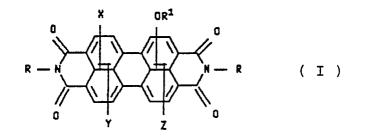
wherein each R, individually, is substituted or unsubstituted aliphatic, aromatic or heterocyclic radical, X,Y, and Z are, individually, chlorine fluorine, bromine or OR<sup>1</sup> and R<sup>1</sup> is a substituted or unsubstituted phenyl,
