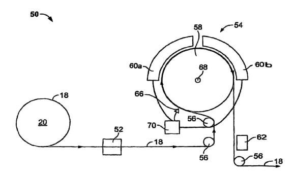
(57) Abstract: A printing system includes a printer that prints only a sense mark on a substrate and an imaging unit. The imaging unit prints data onto the substrate and includes a plurality of printheads. The printing system also includes a sensor that detects the sense mark and a controller that instructs the imaging unit to print data onto the substrate, wherein the controller distributes print data among the plurality of printheads.
