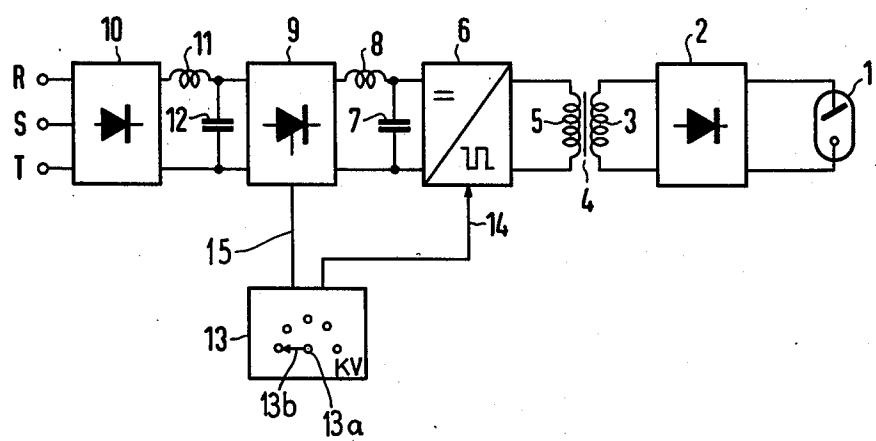
**X-RAY DIAGNOSIS GENERATOR COMPRISING AN INVERTER FEEDING THE HIGH VOLTAGE TRANSFORMER**
