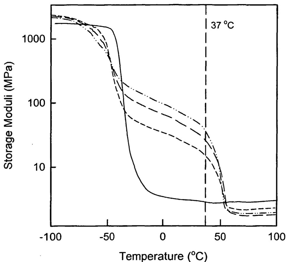
**Figure 7.** Dependence of tensile storage modulus on PCO wt-% in PCO:SBR blends prepared by melt blending and crosslinking with 1 wt-% PCO at  $T = 180$  °C for 30 min.
