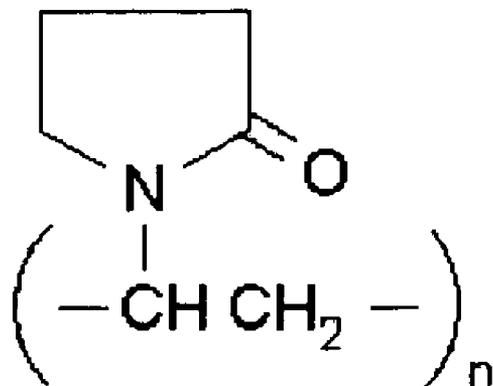
**Figure 9: Molecular structure of PVP**
