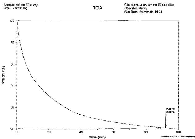
Figure 8: TGA thermogram of amorphous Cefdinir in Eudragit EPO during an isothermal hold at 25°C.
