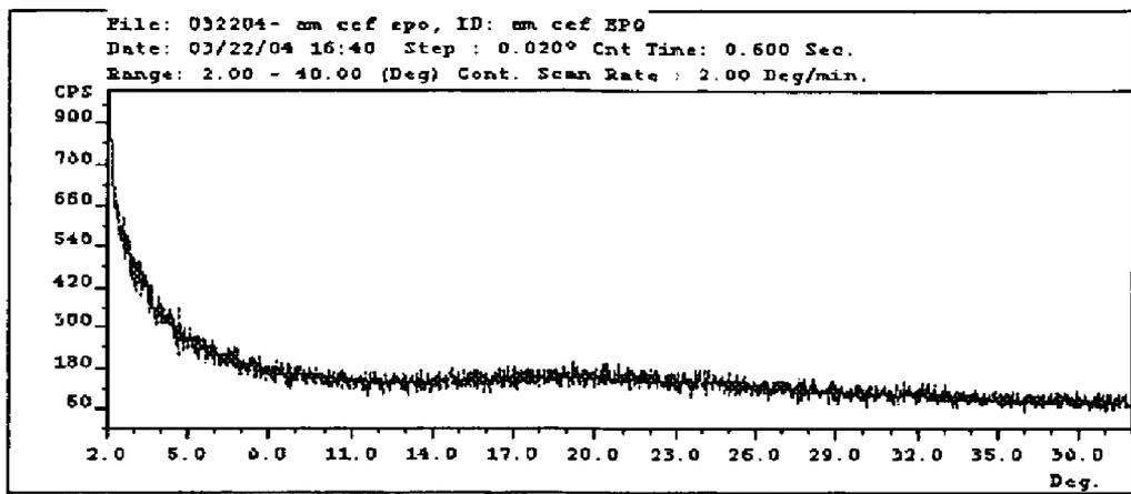
Figure 6: X-ray pattern of amorphous Cefdinir with Eudragit EPO
