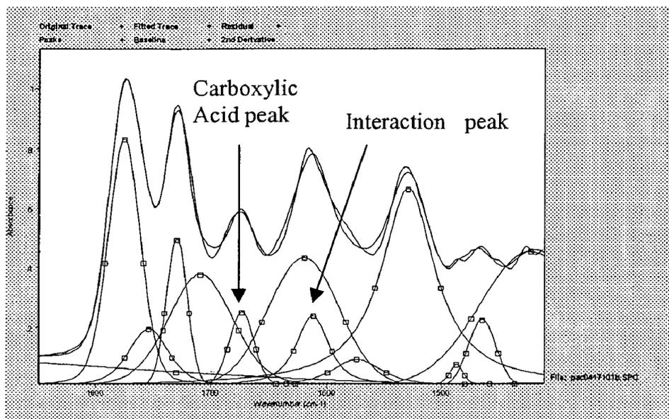
Figure 7b: Fit of Cefdinir/EPO spectra using an additional peak at 1612 cm<sup>-1</sup>
