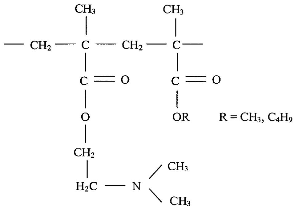
Figure 5: Molecular structure of Eudragit EPO monomer
