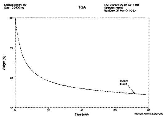
Figure 4: TGA thermogram of amorphous Cefdinir during an isothermal hold at 25°C
