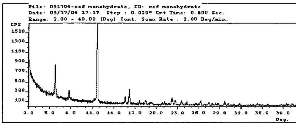
Figure 1: X-ray diffraction pattern for Cefdinir monohydrate
