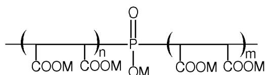
where M is  $\text{H}^+$ ,  $\text{Na}^+$ ,  $\text{K}^+$ ,  $\text{NH}_4^+$ , or mixtures thereof; and the sum of m plus n is greater than 2.
