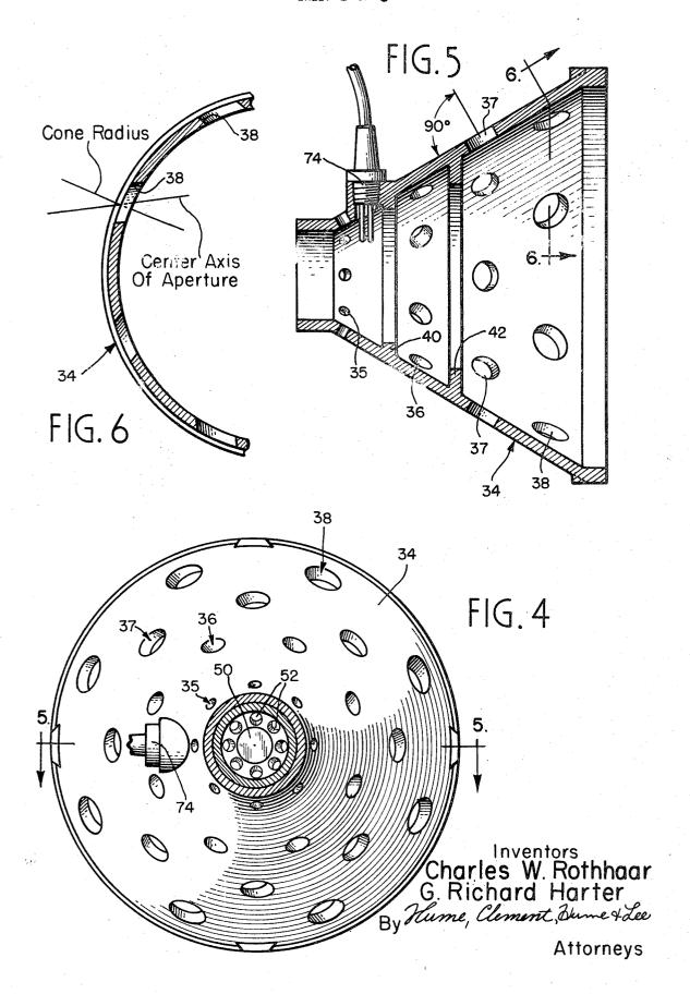
The present invention relates generally to gas burners. More particularly, the invention is directed to a burner of the packaged or self-contained type and to a new and improved 5 gas-air mixing and ignition chamber. Although the burner assembly of the invention is of general utility for air heating and furnace applications, it is particularly suited for use in industrial heating processes and, accordingly, the invention will be described in this latter context.
