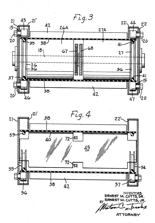
ADJUSTABLE ANGULATED CONVEYOR SYSTEM IN WHICH HOLDDOWN ROLLERS ARE EMPLOYED TO SECURE A RIDGED BELT TO CHANNELED PULLEYS
