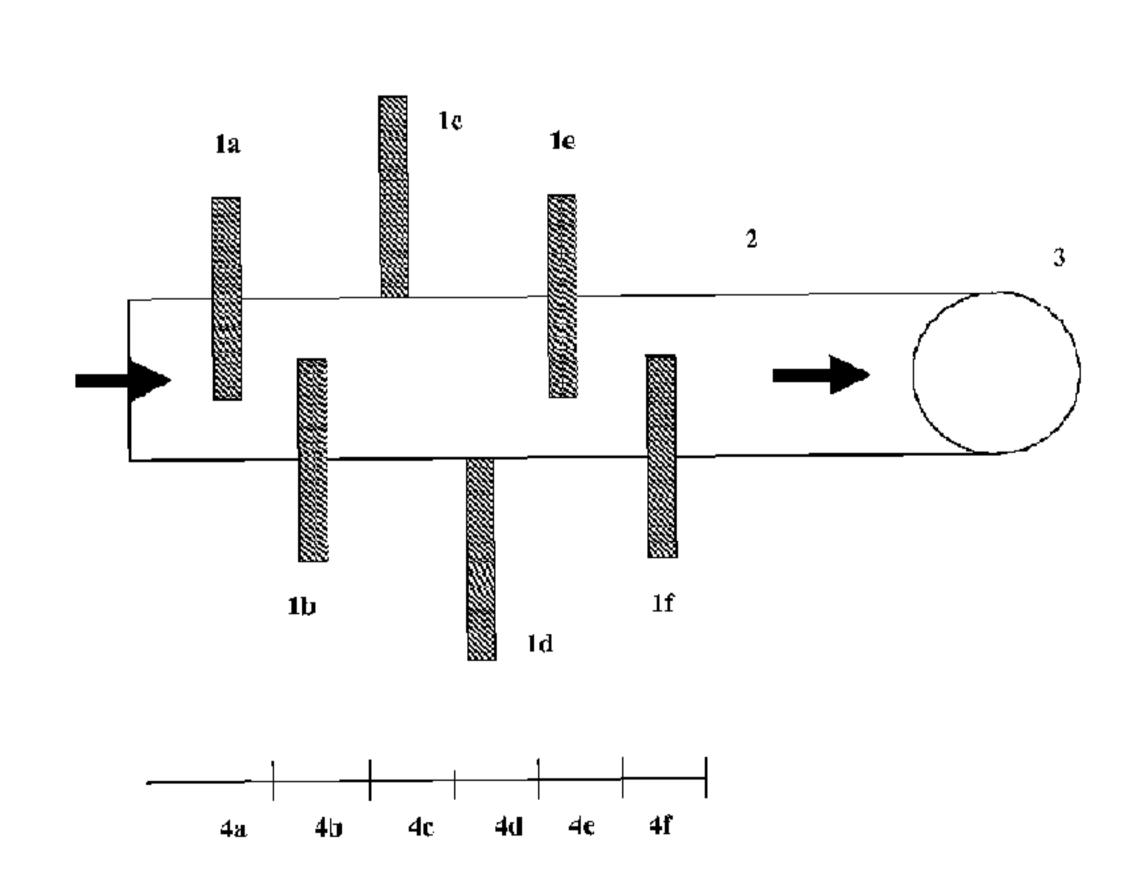
(57) Abstract: Self-cleaning apparatus and methods are disclosed for handling viscous fluids, such as thick solid-liquid slurries of lignocellulosic biomass and its components, under high pressure, using an array of retractable valves.
