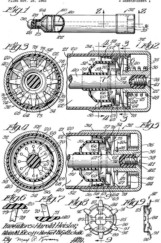
H. HEISLER ETAL CONTAINER AND DISPENSER FOR DISPENSING PREDETERMINED, SET, MEASURED AMOUNTS OF MATERIAL
