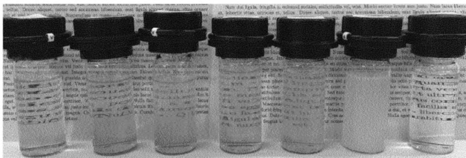
WPI-B WPI-B WPI-B WPI-B WPI-B WPI-B BLG pH 3.0 pH 3.3 pH 3.4 pH 3.5 pH 3.6 pH 3.7 pH3.7
