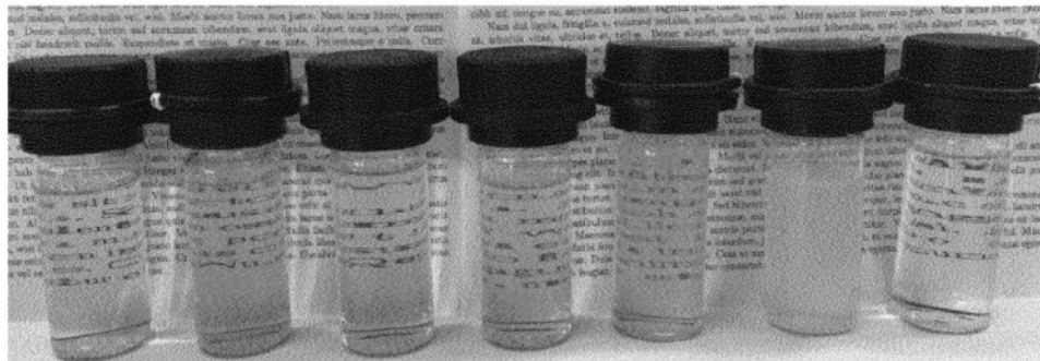
WPI-B WPI-B WPI-B WPI-B WPI-B WPI-B BLG pH 3.0 pH 3.3 pH 3.4 pH 3.5 pH 3.6 pH 3.7 pH3.7
