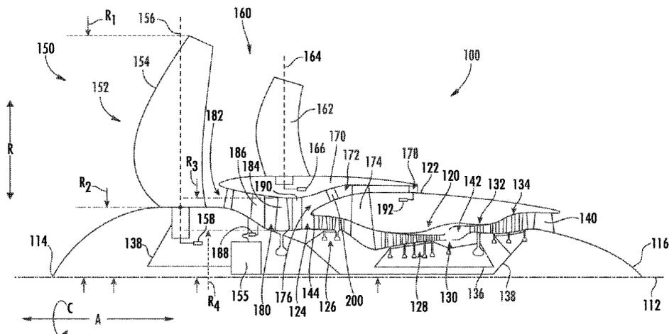
wherein EFP is between 1.5 and 11, wherein  $RqR_{Prim.-Fan}$  is a ratio of  $R_1$  to  $R_2$ , and wherein  $RqR_{Sec.-Fan}$  is a ratio of  $R_3$  to  $R_4$ .
