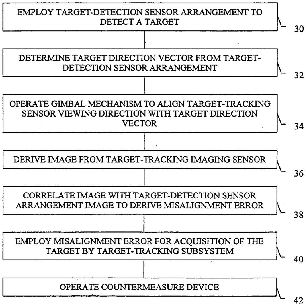
**SYSTEM AND METHOD FOR AUTOMATICALLY ACQUIRING A TARGET WITH A NARROW FIELD-OF-VIEW GIMBALED IMAGING SENSOR**
