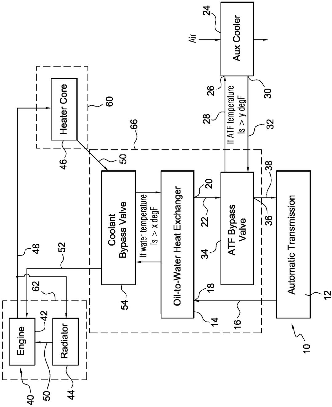
**REGULATING TRANSMISSION FLUID AND ENGINE COOLANT TEMPERATURES IN A MOTOR VEHICLE**
