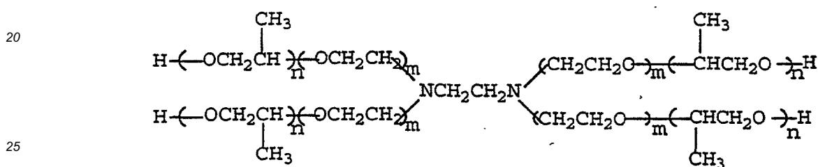
having a number average molecular weight of 8,000 to 20,000 and a ratio of n/m of 8 to 15. The structure may be either linear triblock (ABA or BAB) morphology in which A represents polyethylene oxide and B the polypropylene oxide.
