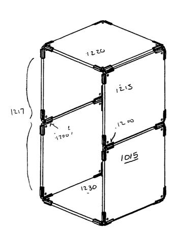
(57) Abstract: A snap together connection system whereby panels or other elements can be connected to form structures. Catches snap into latches thereby connecting panels or other elements. Snap in straight connectors may be used as a bridge to connect panels or other elements in-line.
