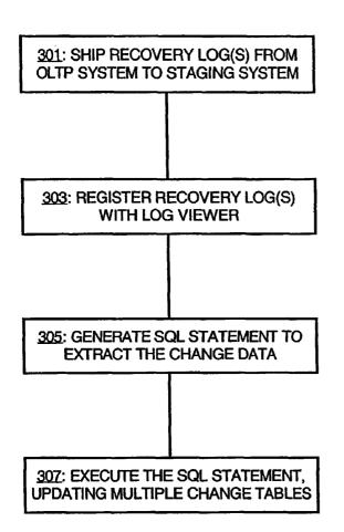
(57) Abstract: A method and software for change data capture is described, in which change data is extracted from a recovery log in a single pass and stored into multiple database objects, such as change tables. The change data indicates modifications that has been performed to multiple source objects that correspond to the multiple database objects. In a preferred embodiment, this can be accomplished with a single multi-table insert SQL statement.
