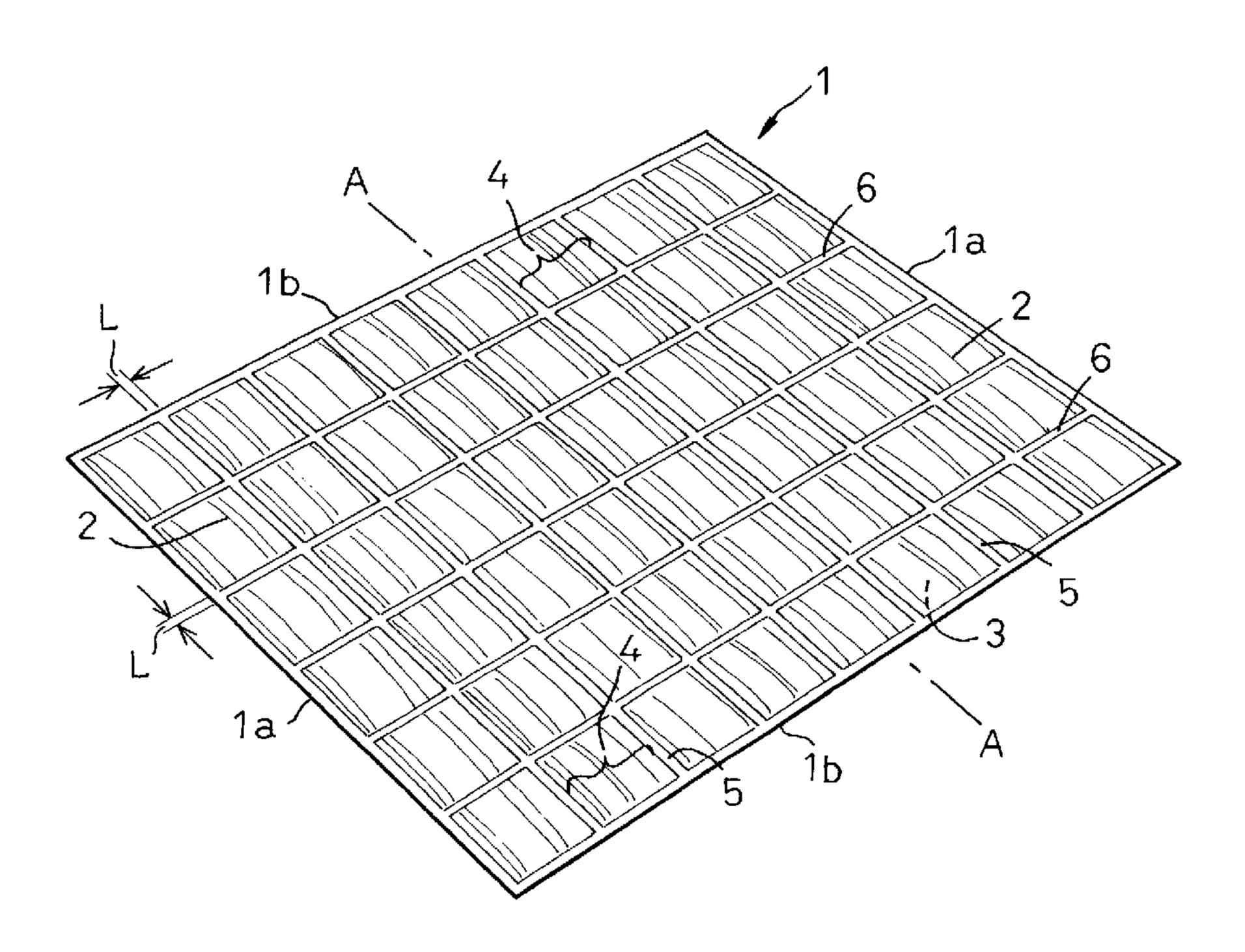
(57) A mechanical fastener including a loop member 1 includes a base sheet 3 and a plurality of continuous filaments 2 extending substantially parallel one to another on one surface of the base sheet 3 substantially parallel one direction and the filaments 2 are bonded to the base sheet 3 along at least a pair of bonding zones 5, 6 extending transversely of the filaments 2 to form a plurality of loop elements 4a extending between the pair of bonding zones 5, 6.
