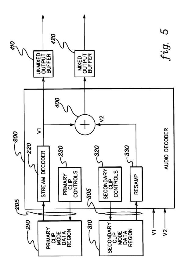
FACILITY FOR SIMULTANEOUSLY **OUTPUTTING BOTH A MIXED DIGITAL** AUDIO SIGNAL AND AN UNMIXED DIGITAL AUDIO SIGNAL MULTIPLE CONCURRENTLY RECEIVED STREAMS OF **DIGITAL AUDIO DATA**
