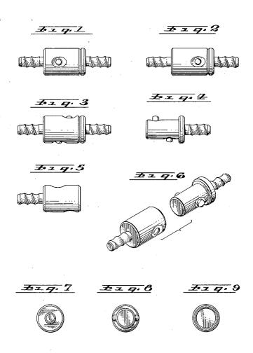
FIG. 1 is a top plan view of an assembled snap coupling showing my new design;
