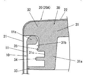
direction, is in close contact with the inner peripheral surface of the container body, while the outer peripheral portions of other ring-shaped protrusions are radially separated from the inner peripheral surface of the container body.
