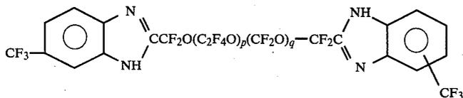
having a molecular weight of 3750 and a p/q ratio of 0.7, synthesized by stoichiometric reaction, at 150° C. in a nitrogen atmosphere, from the corresponding methyl diester and from 3,4-diaminobenzotrifluorine.
