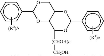
(57) **Abstract**: A tire has a tread which comprises a rubber composition. The rubber composition is based on at least a diene elast-omer, a reinforcing filler, a plasticizing agent comprising between 10 and 60 phr of a polar liquid plasticizer, and a diacetal represented by the formula (I).
