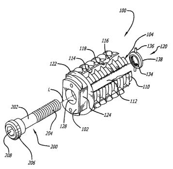
(57) Abstract: Interbody spinal fusion implants (100) being at least in part radially expandable at one of the leading (104) or trailing (102) ends to expand both the height and at least a portion of the width of the implant (100). Instruments (300) and methods for inserting the implants (100) into an implantation space in the spine are disclosed.
