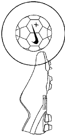
2: Ball comes near and switch is pulled up to strike contact showing proximity to ball
