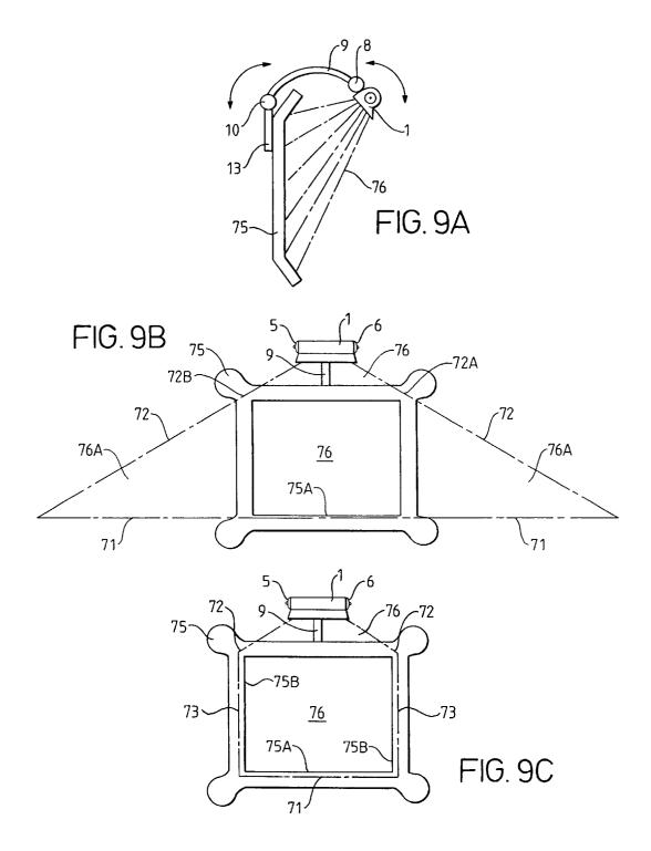
This invention relates to picture lights of the type that have a fitting at one end which can be mounted on the picture or wall with an arm extending forwardly therefrom having a light at its remote end whose beam can be directed onto the
