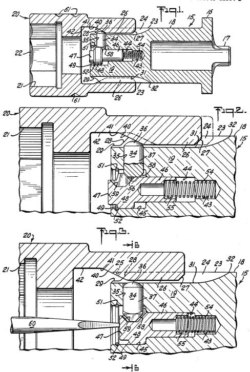
SOCKET CONNECTING MEANS FOR A ROTARY IMPACT TOOL
