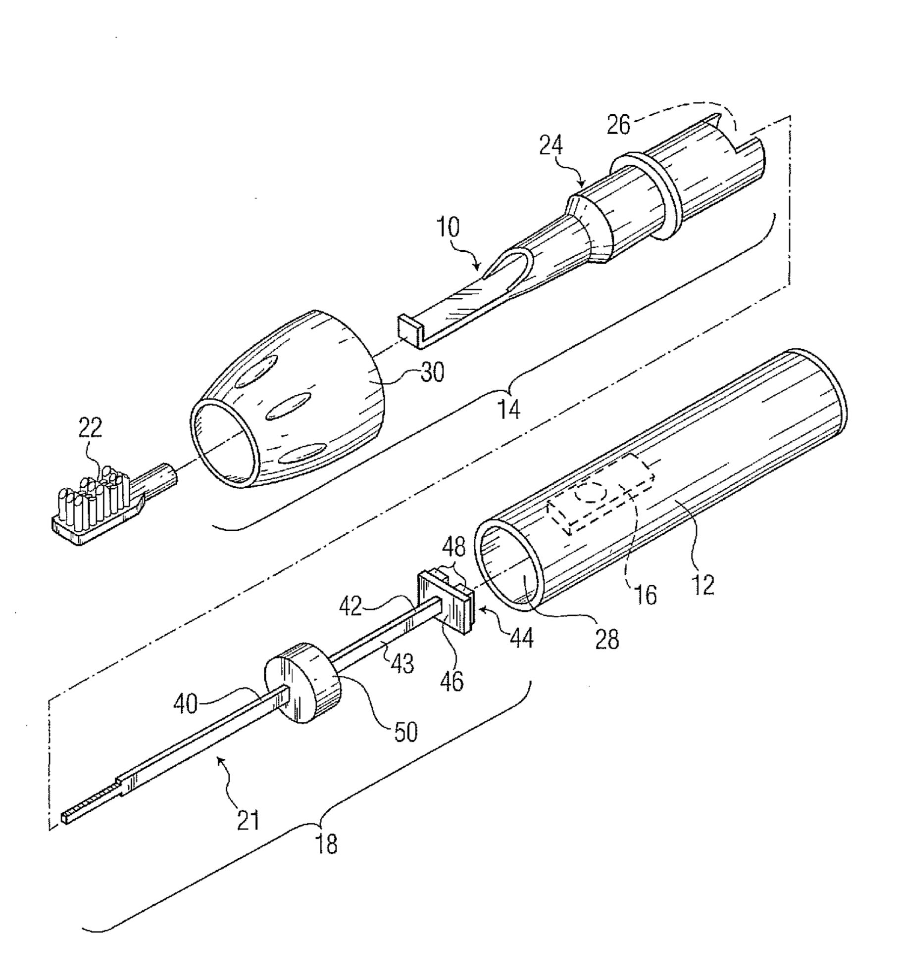
(57) Abstract: The resonator assembly for a power toothbrush includes an elongated solid from stainless rod made steel, having a back assembly which includes permanent magnets which interact with an electromagnet in a drive system in the handle of the toothbrush to produce a transverse motion of the rod. A mount member is connected to the rod at a selected point along its length, and is mounted to a toothbrush housing so that the rod resonates about the mount member at a selected frequency.
