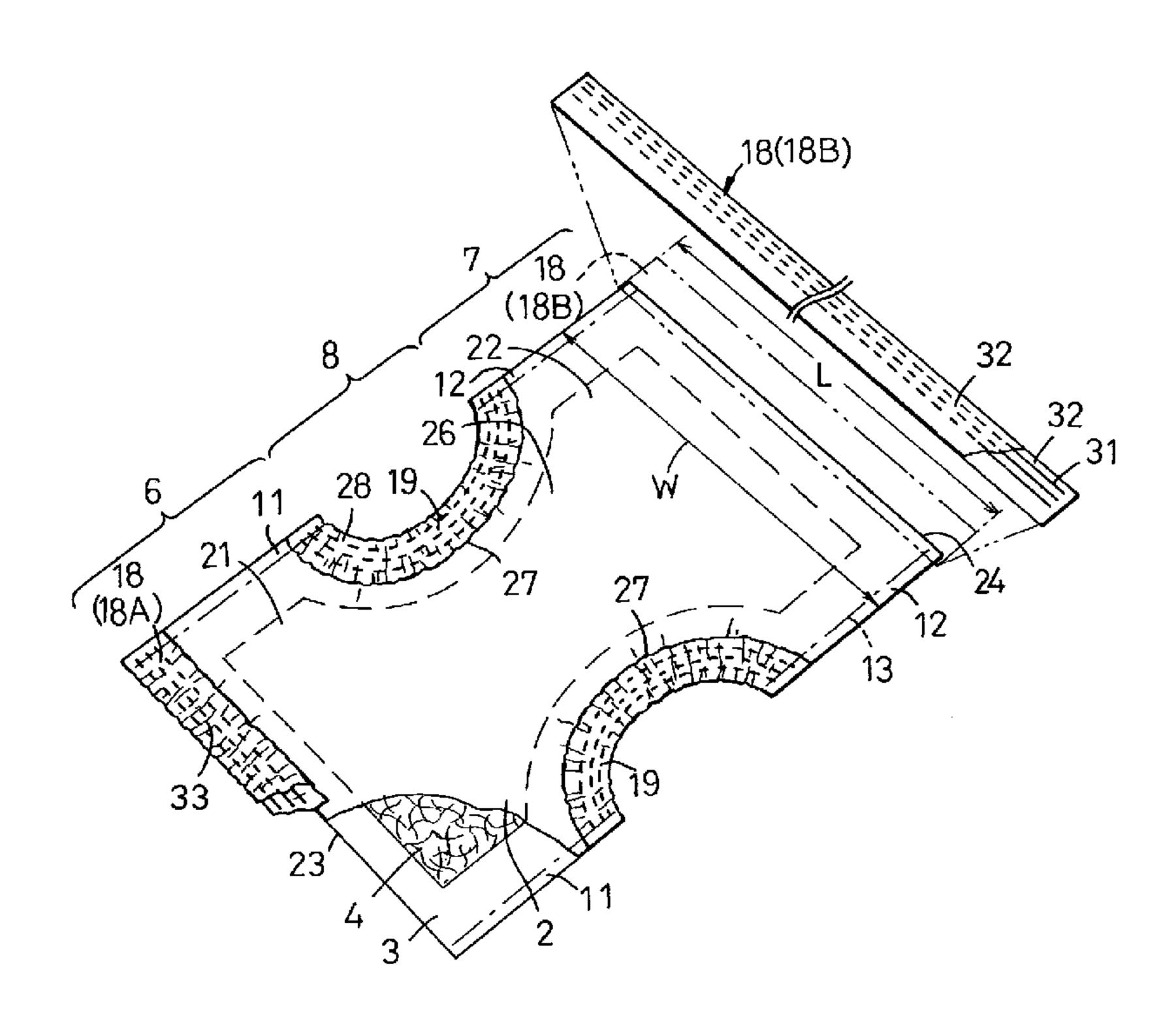
(57) Front and rear waist regions 6, 7 of a diaper 1 having a waist-hole 16 of which a peripheral edge is elastically stretchable in a circumferential direction respectively include covering zones 21, 22 and elastic zones 18A, 18B adapted to be stretchable beyond lengths of the covering zones 21, 22 in the circumferential direction.
