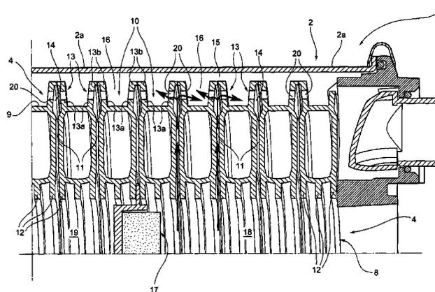
gases which during use pass through the interspaces (11, 14) between the turns of the helical conduit (8).
