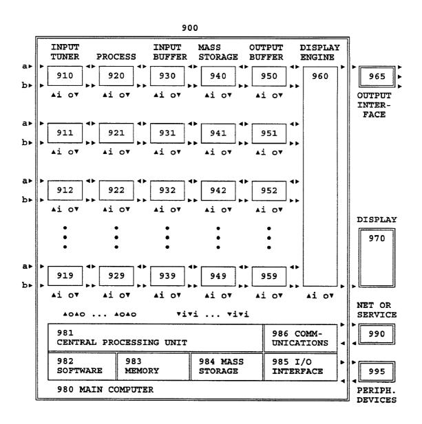
FIGURE 9A: SYSTEM DIAGRAM OF SETTOP BOX OR OTHER DEVICE
