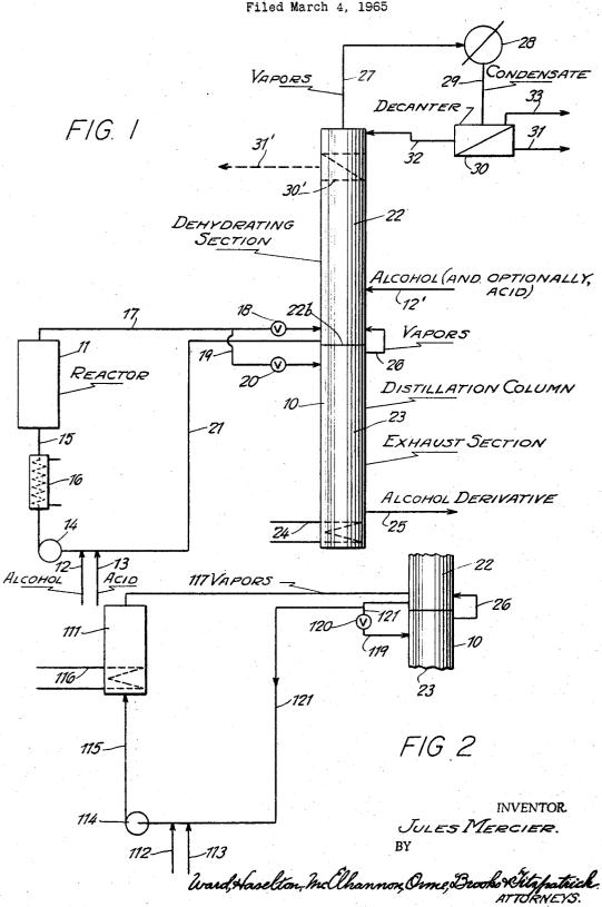
3,404,175 PROCESS FOR FORMING AND SEPARATING ETHERS OR ESTERS BY PLURAL STAGE DIS-TILLATION WITH REMOVAL OF WATER AS AN AZEOTROPE
