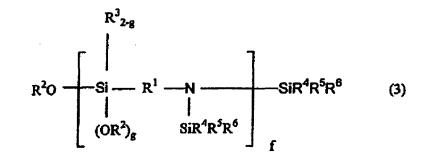
wherein  $R^1$ ,  $R^2$ , and  $R^3$  have the same meanings as defined for the formula (1),  $R^4$ ,  $R^5$ , and  $R^6$  individually represent an alkyl group having 1 to 20 carbon atoms or an aryl group or two of  $R^4$ ,  $R^5$ , and  $R^6$  may bond to form a ring together with the silicon atom to which  $R^4$ ,  $R^5$ , and  $R^6$  bon, g is 1 or 2, and f is an integer from 1 to 10, or the following formula (4),
