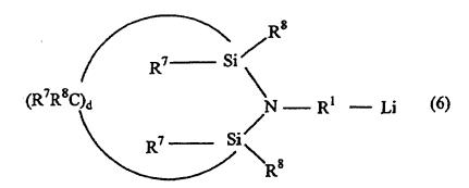
**[0077]** wherein R<sup>1</sup> has the same meaning as defined for the formula (3), R<sup>7</sup> and R<sup>8</sup> individually represent a hydrogen atom, an alkyl group having 1 to 20 carbon atoms, or an aryl group, and d is an integer from 1 to 7, and at the time when the polymerization is substantially completed, an alkoxysilane compound shown by the following formula (7), **[0078]**
