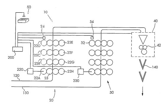
(57) **Abstract:** A method for presetting motor phase in a web printing press includes providing a mark (70, 72) on a printing form (122), the mark being a function of a desired preset phase for a motor (220, 230) driving the printing form during printing. The mark is read using a sensor (24, 34), the sensor having a sensor output. The phase of the motor is preset as a function of the sensor output. A printing form and web printing press are also provided.
