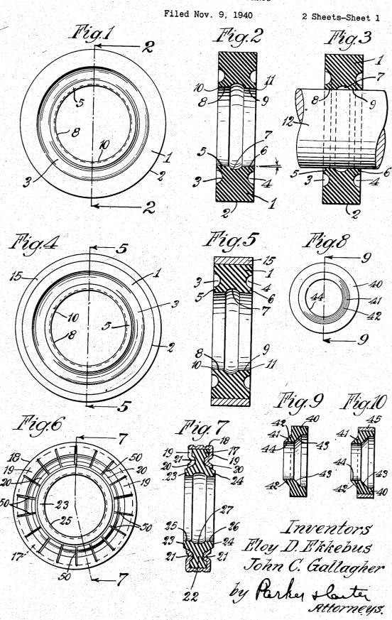
OIL SEAL FOR MOVING PARTS
