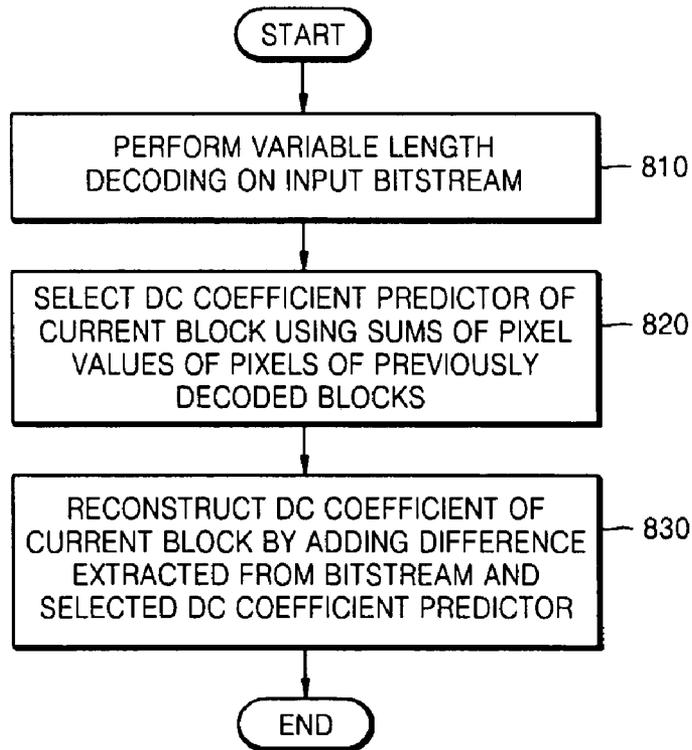
**METHOD OF AND AN APPARATUS FOR PREDICTING DC COEFFICIENT IN TRANSFORM DOMAIN**
