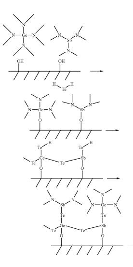
**[0029]** As more thermally stable tellurium compounds, organotellurols and deuterated organotellurols are disclosed as more suitable tellurium precursors for ternary germanium-antimony-tellurium film depositions.
