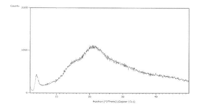
Figure I shows a powder X-ray diffraction pattern of the amorphous Trisodium Sacubitril Valsartan complex.
