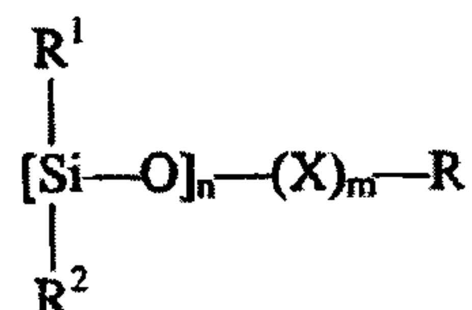
wherein  $\text{R}^1$  and  $\text{R}^2$ , independently, are an alkyl group having 1 to 8 carbon atoms, or an unsubstituted or substituted aromatic group having 6 to 10 carbon atom,  $\text{X}$  is a functional group independently selected from substituted or unsubstituted OH,  $\text{OR}^3$ ,  $\text{N}(\text{R}^4)_2$  enoxy, acyloxy, oximo, and aminoxy, wherein  $\text{R}^3$  and  $\text{R}^4$  are, independently, an alkyl or cycloalkyl having 1 to 8 carbon atoms,
