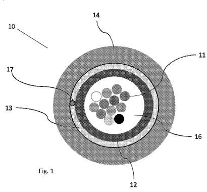
(57) Abstract: The present invention relates to central loose optical-fiber cables. An exemplary optical-fiber cable includes a central buffer tube that encloses loose optical fibers. Stranded strength yarns surround the central buffer tube and the optical fibers positioned within the central buffer tube's annular space, and a cable jacket surrounds the stranded strength yarns.
