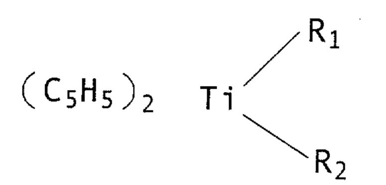
wherein  $R_1$  and  $R_2$  are the same or different and are selected from the group consisting of halogen,  $C_1$ - $C_8$  alkyl and alkoxy groups,  $C_6$ - $C_8$  aryloxy groups, silyl groups and carbonyl groups.
