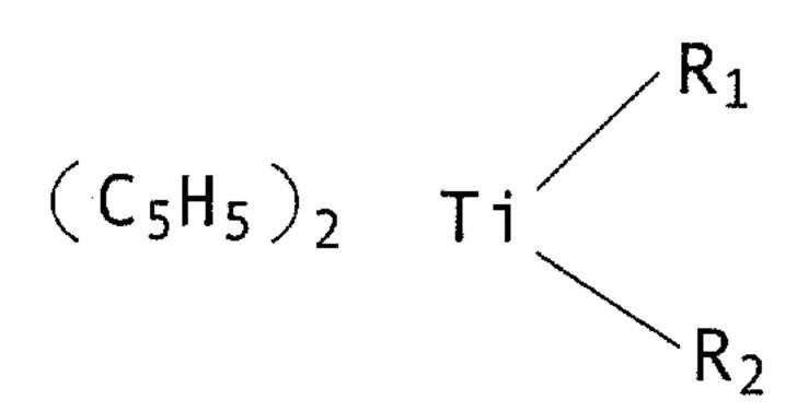
wherein  $R_1$  and  $R_2$  are the same or different and are selected from the group consisting of halogen,  $C_1$ - $C_8$  alkyl and alkoxy groups,  $C_6$ - $C_8$  aryloxy groups, silyl groups and carbonyl groups.
