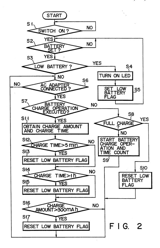
METHOD AND APPARATUS FOR BATTERY CONTROL
