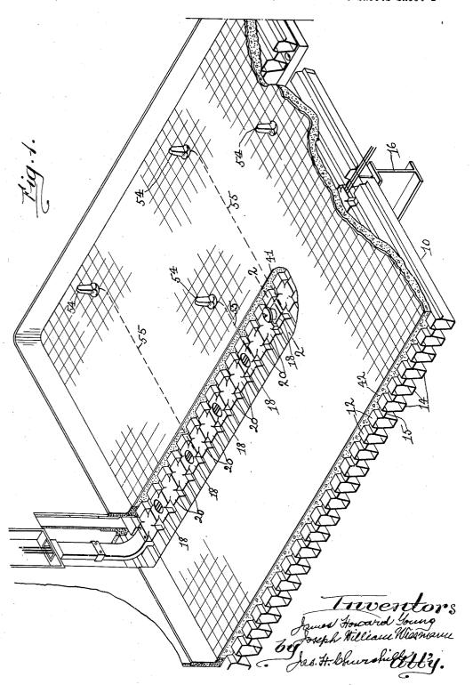
CROSS-OVER DUCT FOR MULTICELLULAR STRUCTURES
