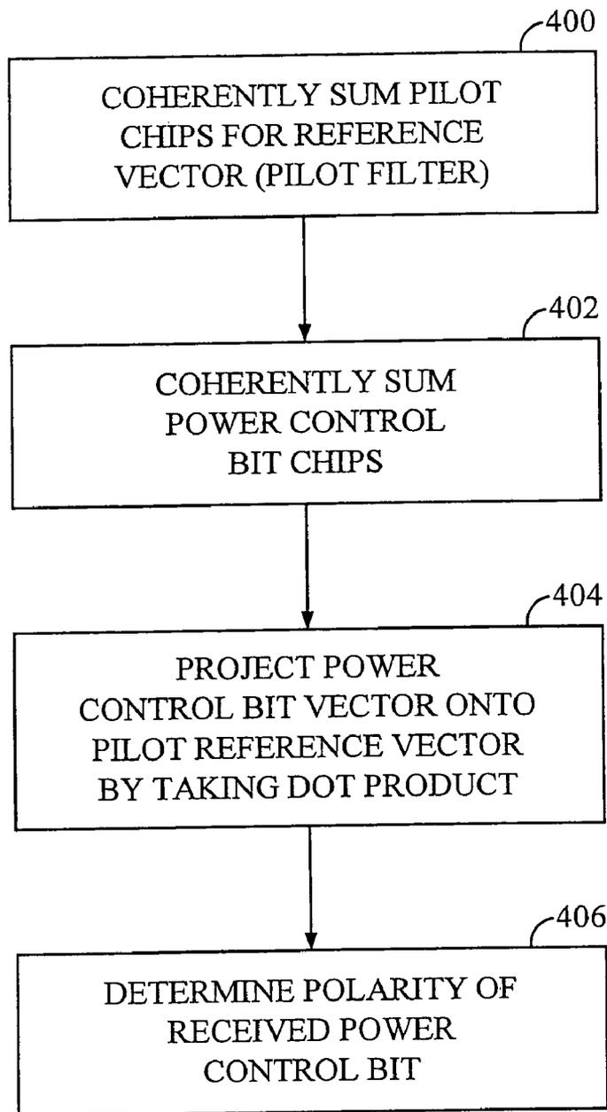
POWER CONTROL BIT POLARITY DETERMINATION METHOD
