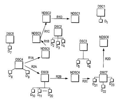
(57) Abstract: A system and method for controlling devices that are part of a peer to peer network of controllers is provided. Messages are routed to controllers of the network and such messages are used to control devices coupled to said controllers. Status messages indicating the state of devices are routed to controllers to allow the state of the devices to be displayed by said controllers.
