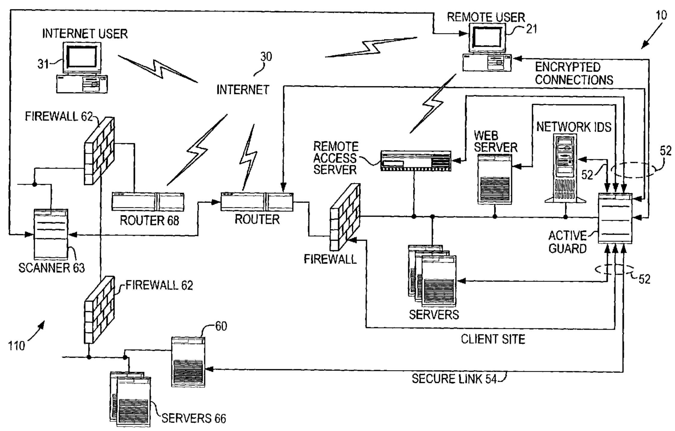
(57) Abstract: A method and apparatus for verifying the integrity of devices on a target network (100) having two components: a subsystem (50) connected to the target network (100), and a master system (60), isolated therefrom by a secure lin (52). The topological and hierarchical relationship of the devices to each other improves stability of the apparatus. Random testing of the subsystem (50) by the master system (60) provide verification and independent self-checking.
