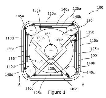
(57) Abstract: A carrier puck (100) for an article of any one of a plurality of different sizes and/or shapes, comprises: a support (105) for supporting the article thereon; and a plurality of locating members (15a, 125b, 125c, 125d) for locating the article between them on the support. A first one of the locating members (125a, 125b, 125c, 125d) is movable so as to reduce a separation distance between it and another one of the locating members.
