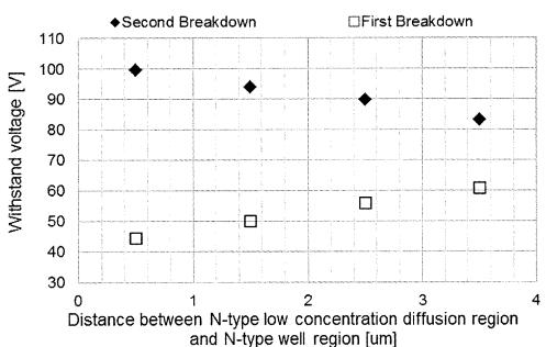
Dependence on distance between N-type low concentration diffusion region and N-type high concentratin drain region
