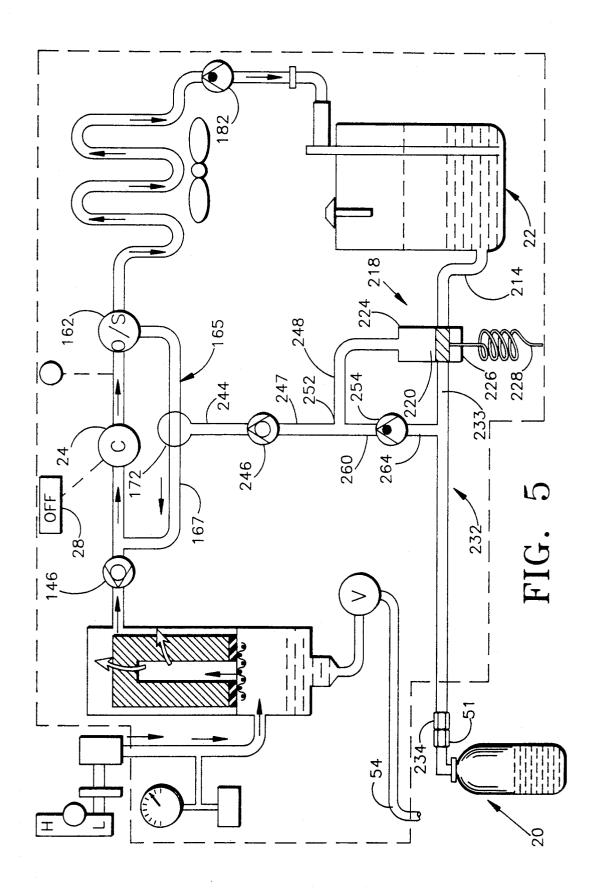
REFRIGERANT RECOVERY DEVICE WITH VACUUM OPERATED CHECK VALVE
