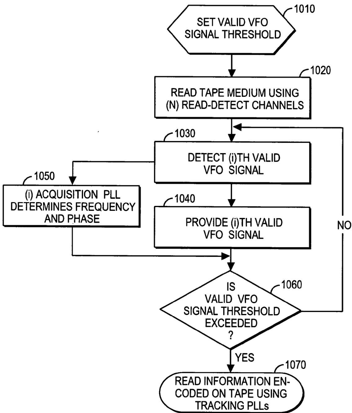
**APPARATUS AND METHOD TO READ INFORMATION FROM A TAPE STORAGE MEDIUM**
